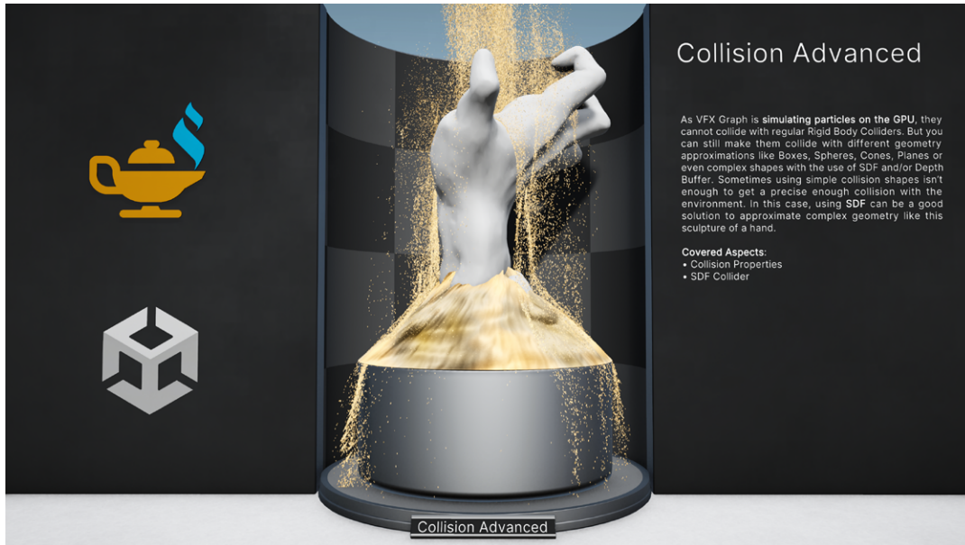
Signed distance fields can approximate complex geometry for collisions.
