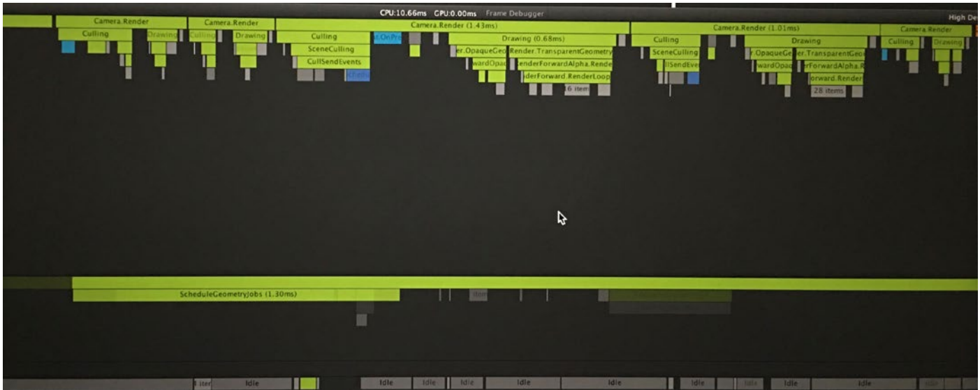
The Unity CPU Profiler shows the main thread in the timeline view and indicates that there are multiple Cameras. Unity performs culling for each Camera.
